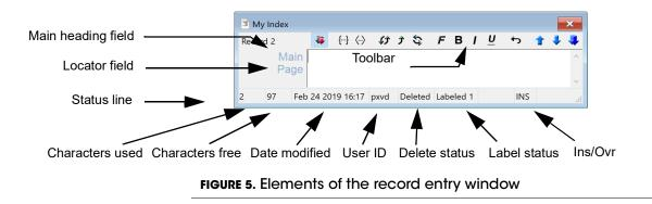
The record entry window is divided into three parts: at the top, a row of buttons, in the middle, an area where you type the entry; at the bottom, a status line. The status line shows, at left, the number of characters already in the record, followed by the number of characters you can add to it. After you have added the record to the index the status line will also show the date and time at which the record was last modified. Sometimes Cindex displays additional status information.
